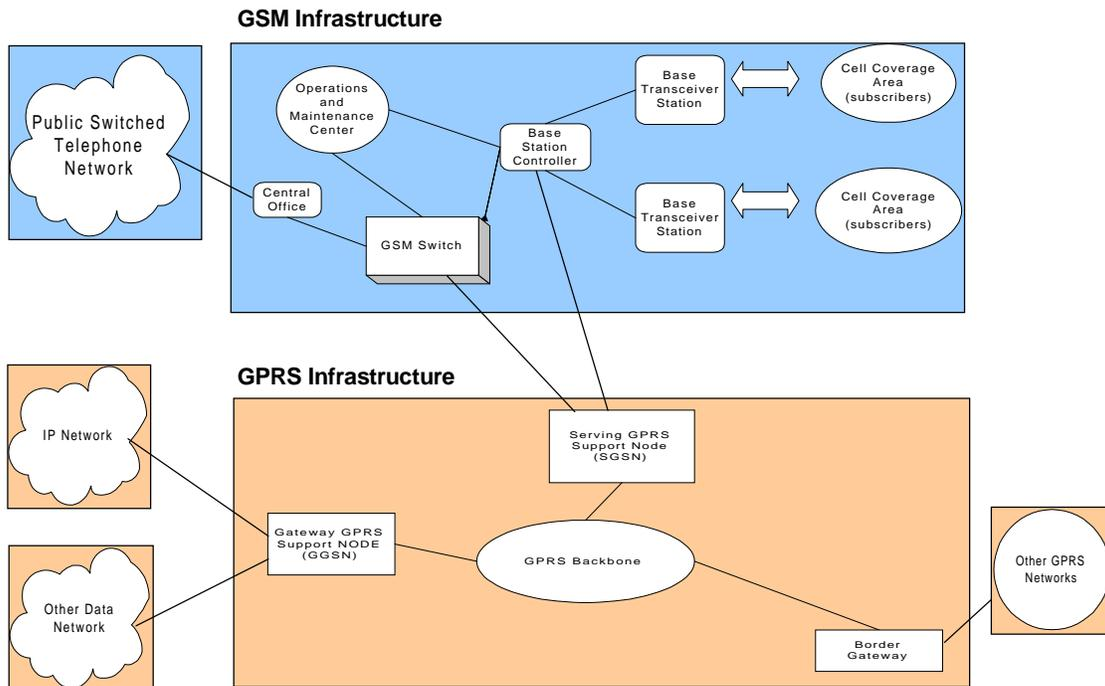
The subscriber logs on to the network separately for GPRS and establishes a Packet Data Protocol (PDP) which is a logical connection between the subscriber and the GGSN via the SGSN. In this manner, a GSM subscriber is able to directly access data networks such as the Internet without the necessity of a modem.
